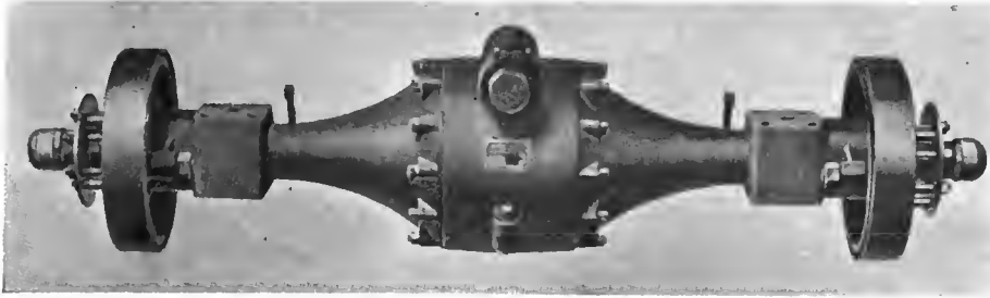
The new 1-ton worm-driven axle made by the Empire Axle Co., Dunkirk, N. Y. It is characterized by the fact that it has no differential and is the first stock axle to be so offered on the market in this country. The housing is of the three-piece type, following previous Empire practice. The central part of the housing carries the worm and wheel as a complete unit
